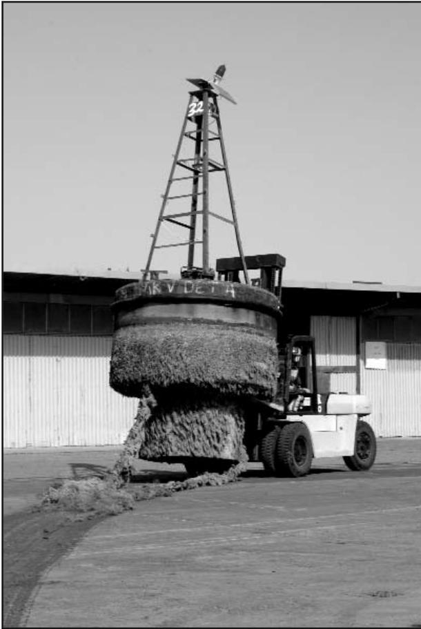
**Figure 5.** Aged Iraqi buoy showing marine growth encrustation and dilapidated upper works. (Coast Guard Collection)
