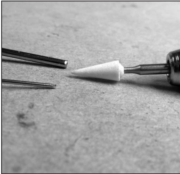
Figure 22. Modified syringe needles and the ceramic stone for fine finishing.
