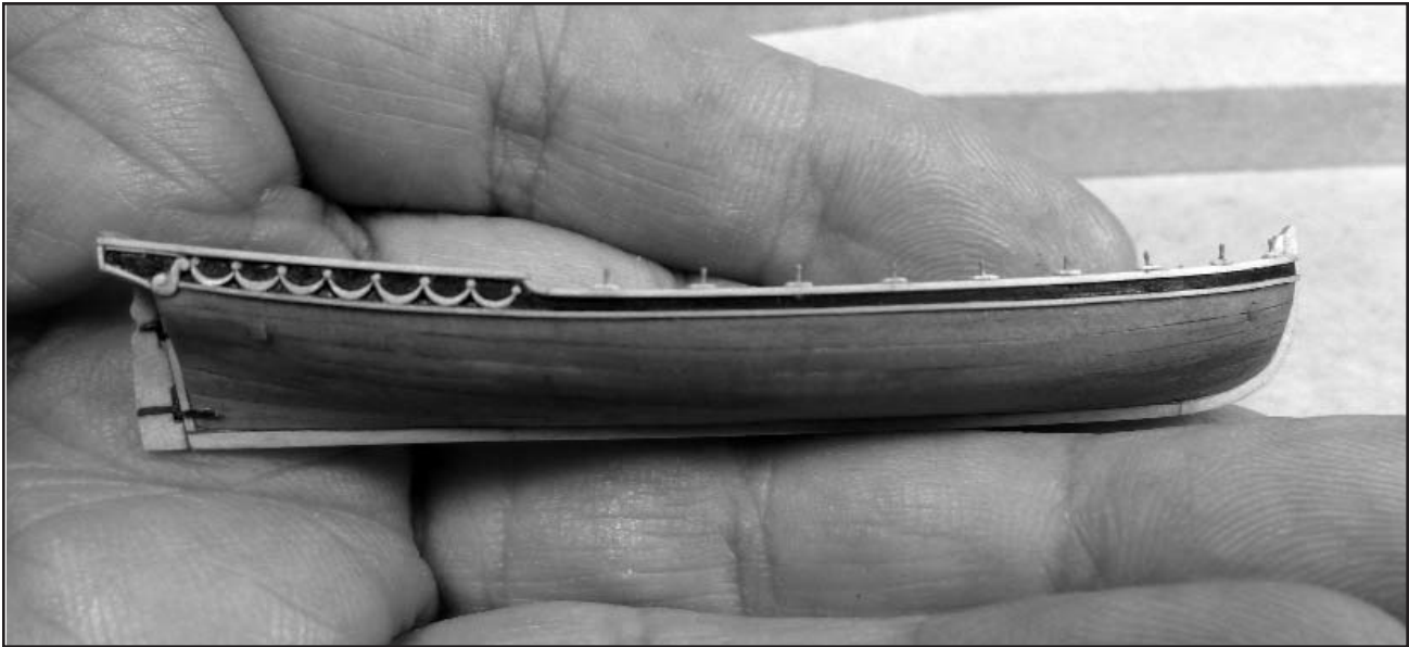
Figure 24. Tholepins in place.
