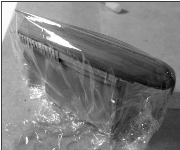
Figure 8. The hull wrapped in clingfilm.
