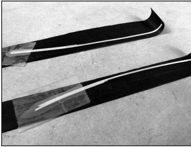
Figure 16. Making washboard laminates of ebony and boxwood.
