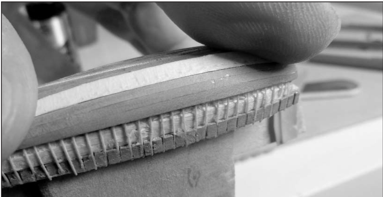
Figure 5. Spiling the final plank.
