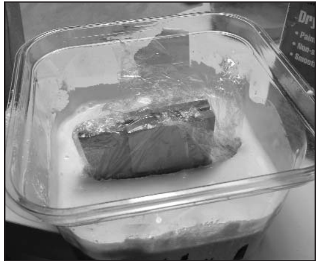
Figure 9. Making the external support mold.
