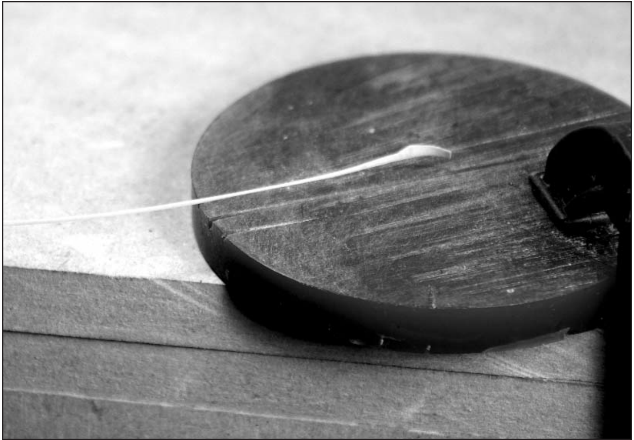
Figure 6. Jeweler's wax holding a plank for finishing.
