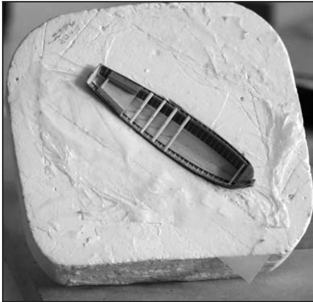
Figure 10. Fitting out the hull in the external support mold.
