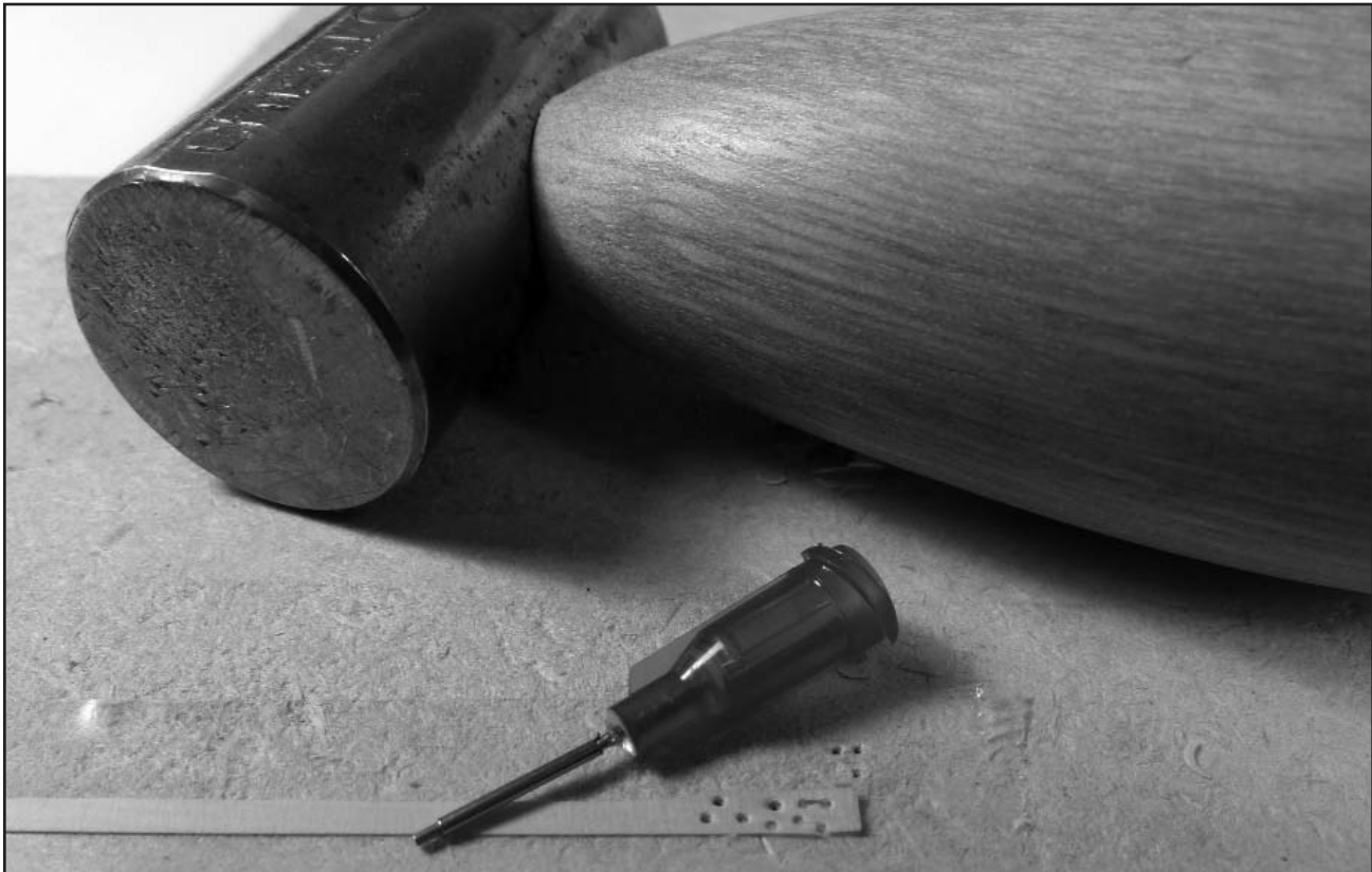
Figure 21. Punching out boxwood for carvings.
