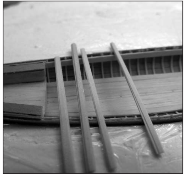
Figure 11. Ceiling planking in place.
