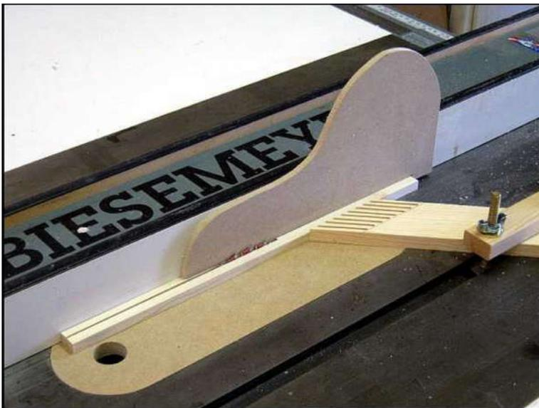
Use the push shoe to guide the stock through the blade.
