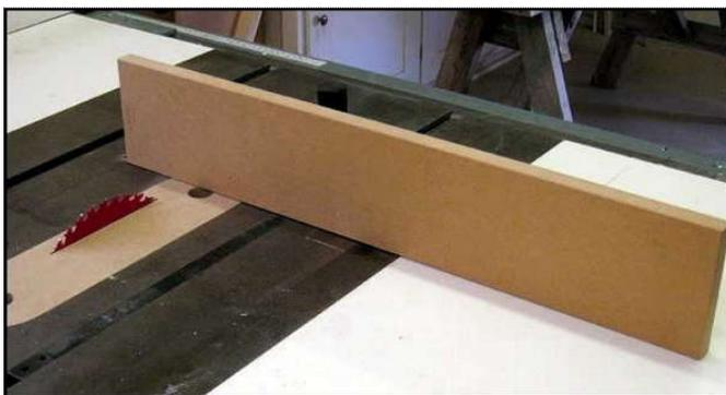
Attach the auxiliary fence to the miter gauge.
