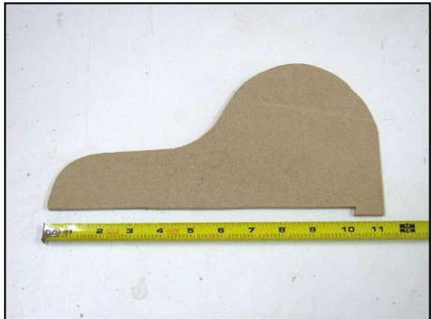
Push shoes are about 12" long and 6" tall. They are made from 1/4" thick hardboard or tempered Masonite.
