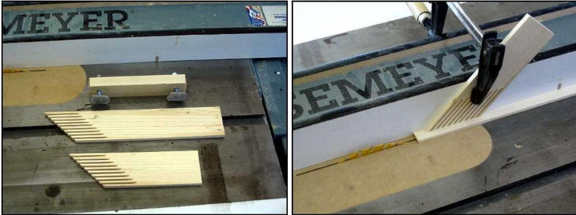
The longer feather board gets clamped to the surface of the saw table. Its job is to hold the stock against the surface of the rip fence. The hold down clamp is made from a block of wood, two standard toilet bolts, two washers, and either two wing or hex nuts. The bolt heads are cut to fit the "T" slot on the saw table. Here's how the feather board clamps to the table. Just a heads-up tip, not all table saws have T-slot miter gauge slots.
