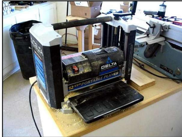
To use a planer, make your "first cut" on the table saw to thickness that's slightly oversized by about 1/16" and finish in the planer. The 1/16" oversize insures you get all of the saw marks out. Make the "second cut" to width on the table saw as shown before. A helper working the out-feed side of the planer is very handy and saves you from a lot of running around both sides of the machine.
