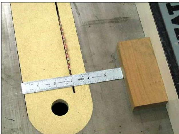
For the first cross cut method, let's cut that 1/4" x 3/8" stock we ripped last time into 3" lengths. Set a nice, clean, squared block of wood against the fence. Set the fence for 3" from the blade to the block.
