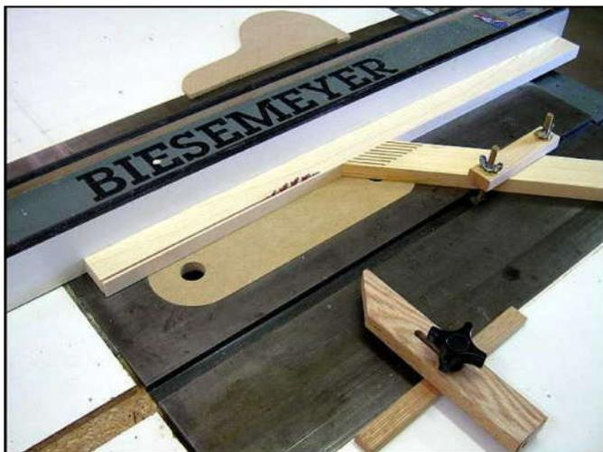
Install, adjust, and clamp down the feather board, making sure that there is enough room left between the tip of the feather board and the saw blade for the nose of the rip fence stop to fit when setting up the next cut. Pull the fence stop out of the miter slot. Then run one of the blank stock pieces through the blade with a push shoe. Check that the resultant strip is exactly 3/32" thick.
