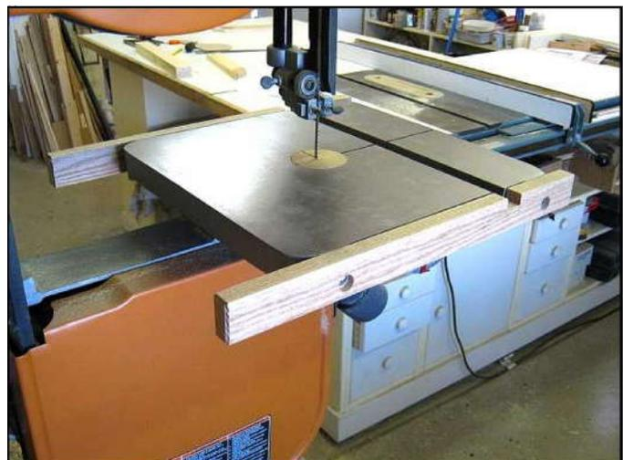
The rails come in handy for any jig or fence you want to clamp to the saw table. The ones I installed here are 18" long.
