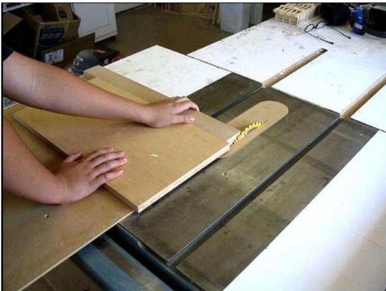
To use the sliding table, hold the panel tight up against the front and push the table through the blade.
