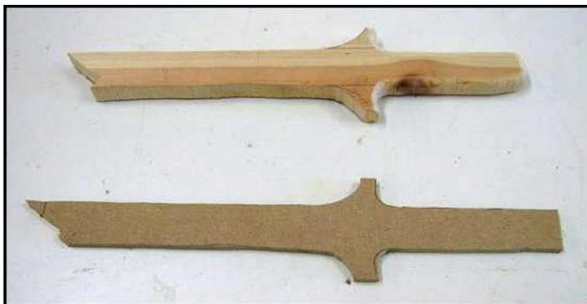
The short stick is for pushing stock through the blade. The longer stick has a notch to help keep stock up against the fence. Here is how they work: Note how chewed up the shorter push stick is. If you don't use a push stick, that's what happens to your fingers. As the sticks wear out replace them. Push sticks are fine to rip bigger lumber, but they are not safe enough to rip thin strips, while cutting scale lumber you'll probably never use a push stick. I don't.
